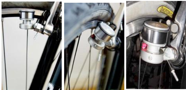
Brake boss adapter left with adjustable ball support, mounting situation, angulation, axis position: Normal position, folded down, working position folded up
