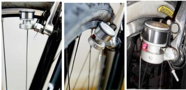
**Brake boss adapter** left with adjustable ball support, mounting situation, angulation, axis position: Normal position, folded down, working position folded up
