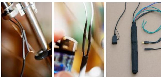
**Cable connection with heat shrink tubing
