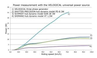
The higher the speed, the more power can be tapped permanently. The 12V output can supply up to 24 W with the maximum current of 2A, enough for extremely bright e-bike headlights. This is OK as a flasher or searchlight, but rather unsuitable as permanent lighting as you would have to drive very fast permanently.
